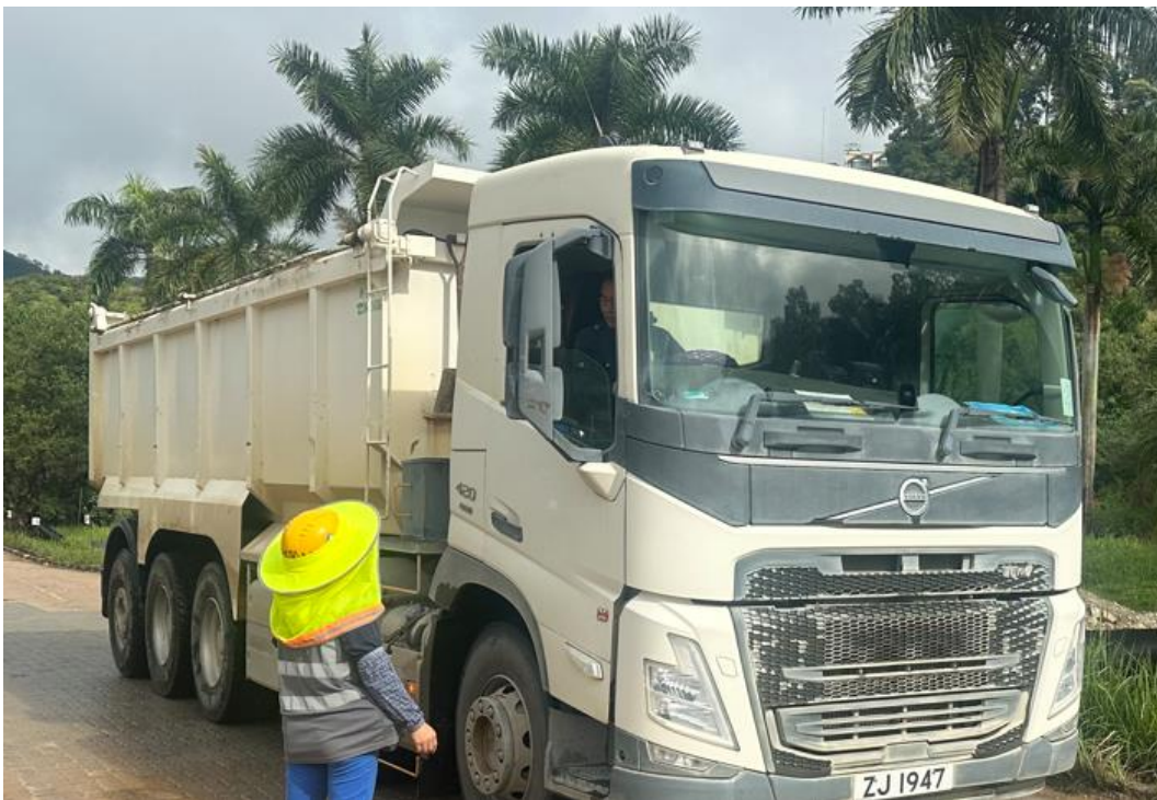
Photo 6 – A worker was assigned to check the wheel condition at site entrance.
